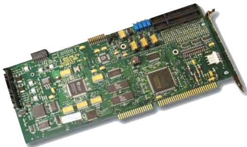
DSP 2 : an enhanced motion control system. The 3000M control is equipped with DSP 2 , an enhanced motion control system that provides significant increases in productivity by producing high speed machining.
