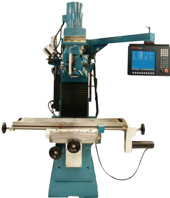
Anilam 3000M 3-axis control with coupled 2-Axis DRO on a Bed Mill
